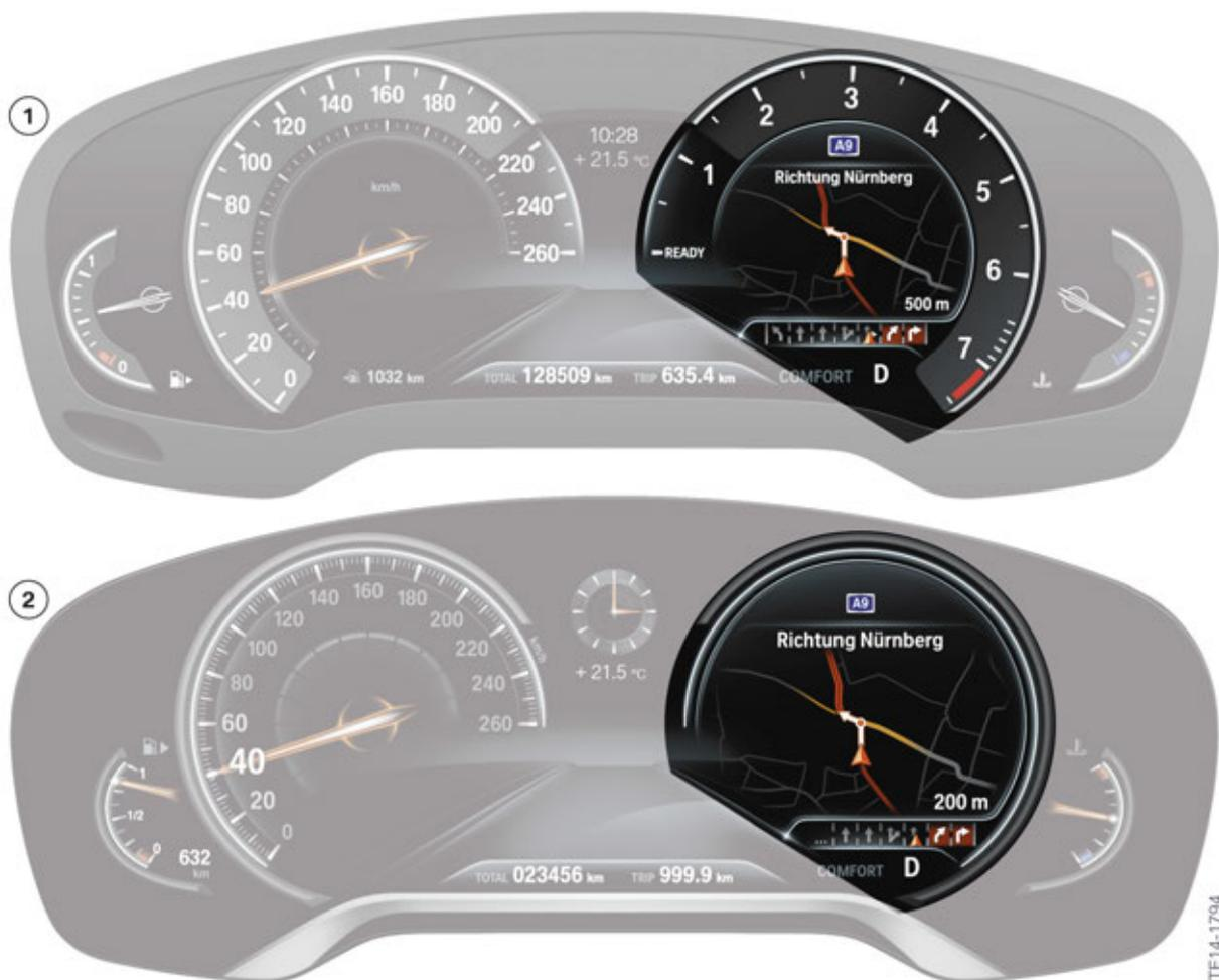
Comparison of the navigation display on the two instrument cluster versions G12
