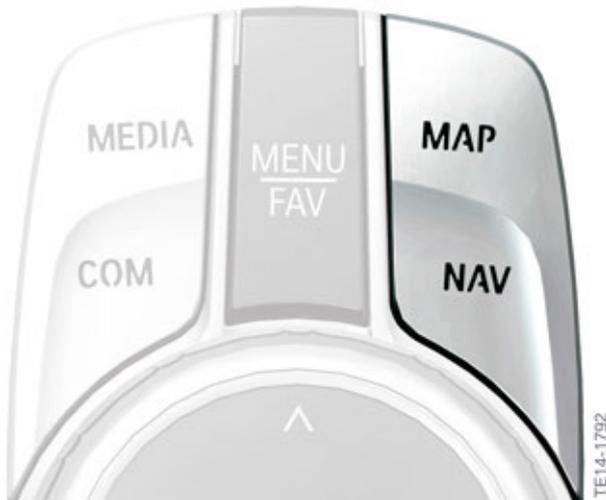
The two direct access keys for the navigation system on the controller
