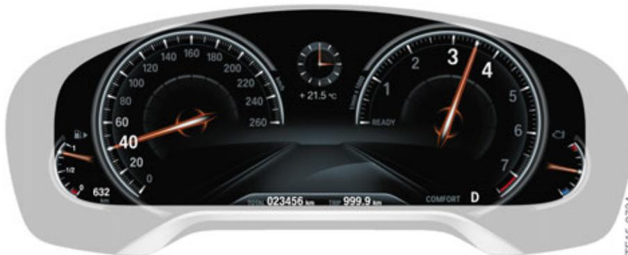
G12 TFT display in the dynamic digital instrument cluster
