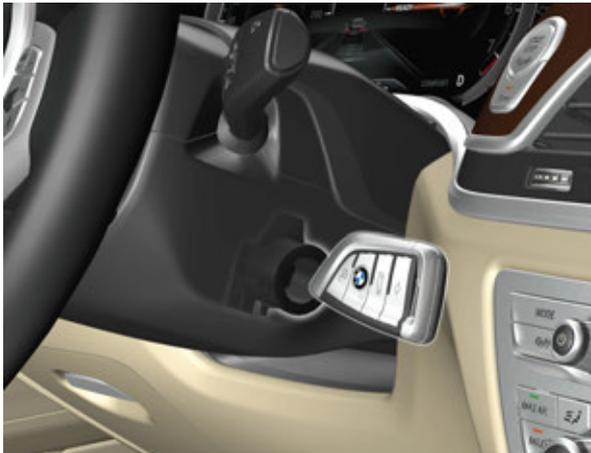
Emergency detection of the remote key
