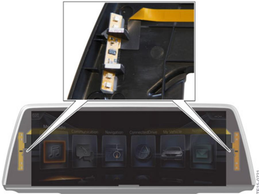
G12 CID including infrared LEDs
