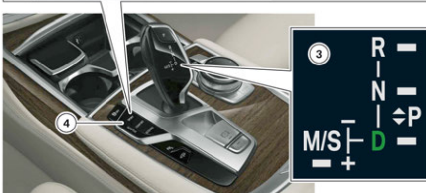
Activation of the additional Sport shift map D + FES Sport in the G12
