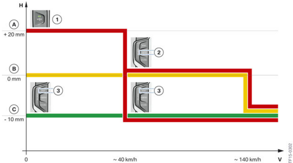
Operating strategy of the air suspension in the G12
