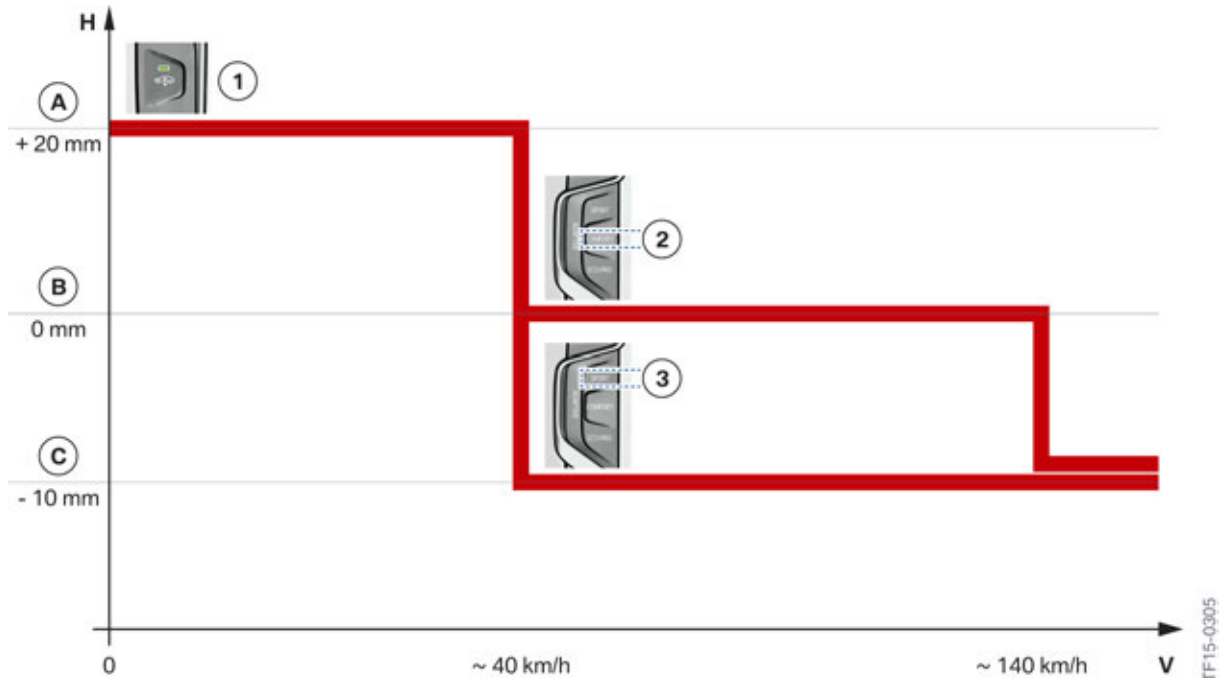
Operating strategy of the air suspension in the G12 at High level
