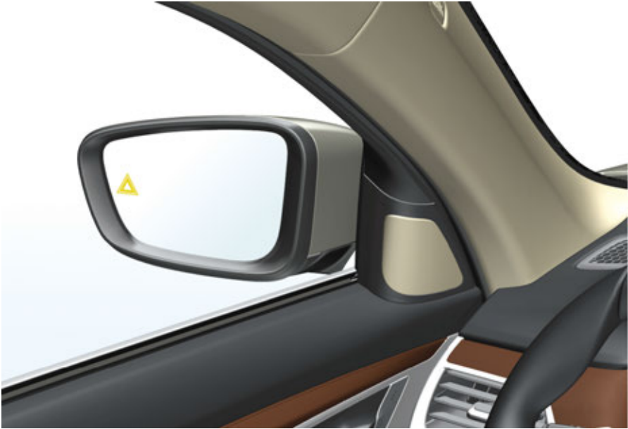
G12 signal unit (LED) in mirror glass
