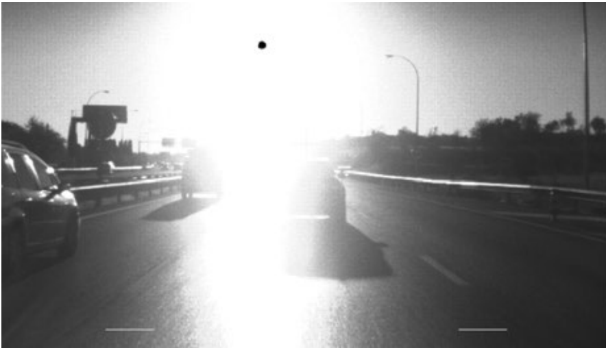
Example of limits of the KAFAS stereo camera
