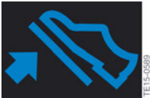
Proactive Active Driving Assistant symbol in the instrument cluster and Head-Up Display
