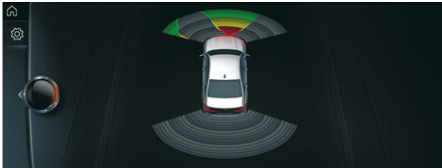
G12 Park Distance Control (PDC) view on the CID
