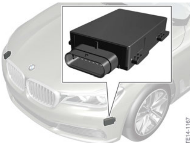
G12 side collision warning (radar sensors)
