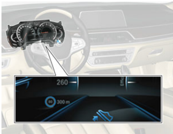
G12 proactive Active Driving Assistant displays in the instrument cluster
