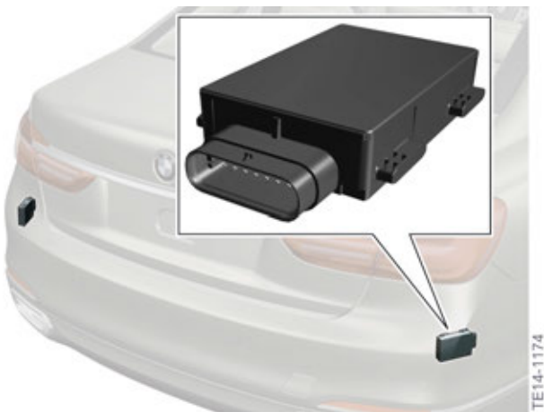
G12 Blind spot detection (SWW) (radar sensors)
