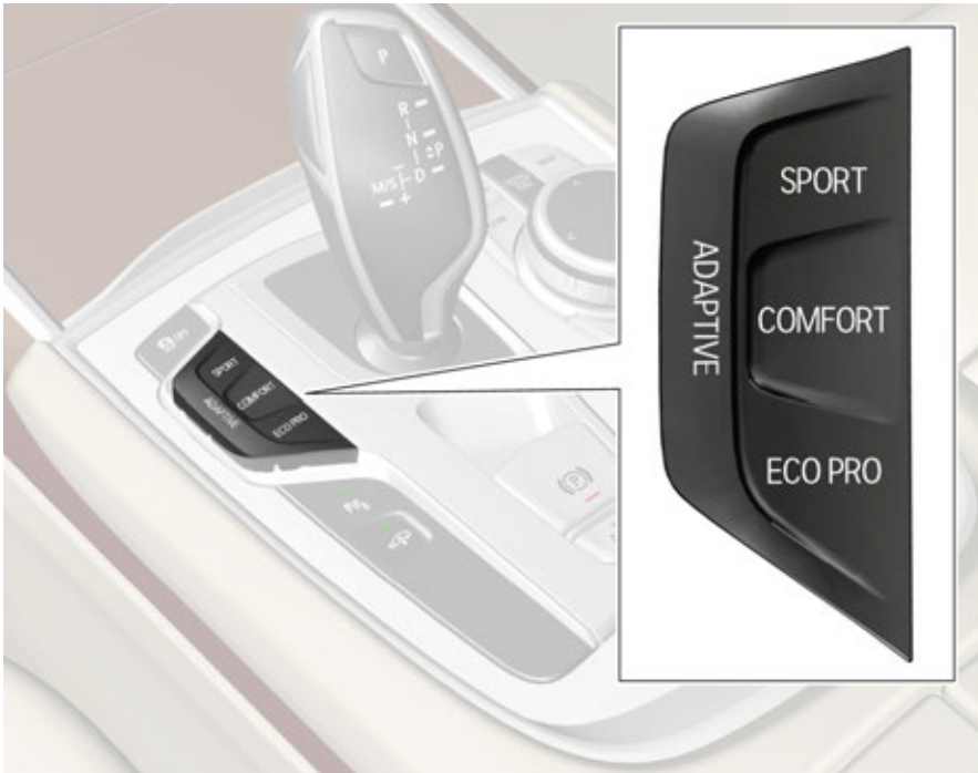
G12 switch block with driving experience switch
