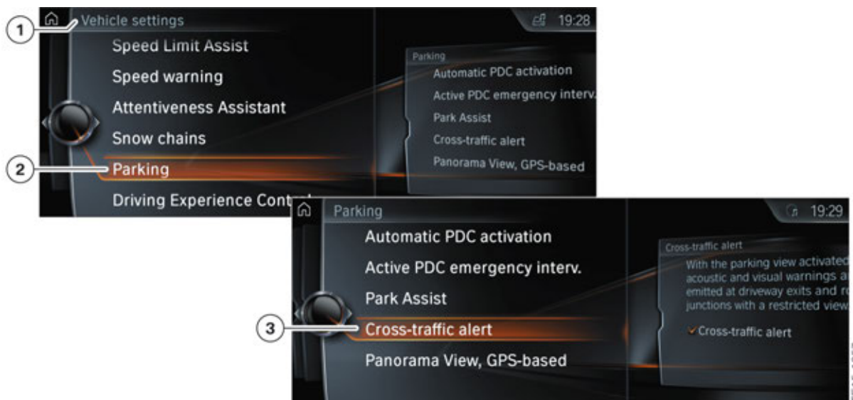
G12 cross-traffic warning activation on the CID
