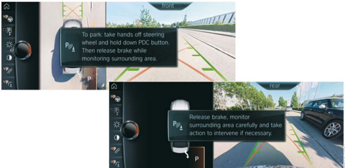
G12 parking procedure using PMA (parallel parking)
