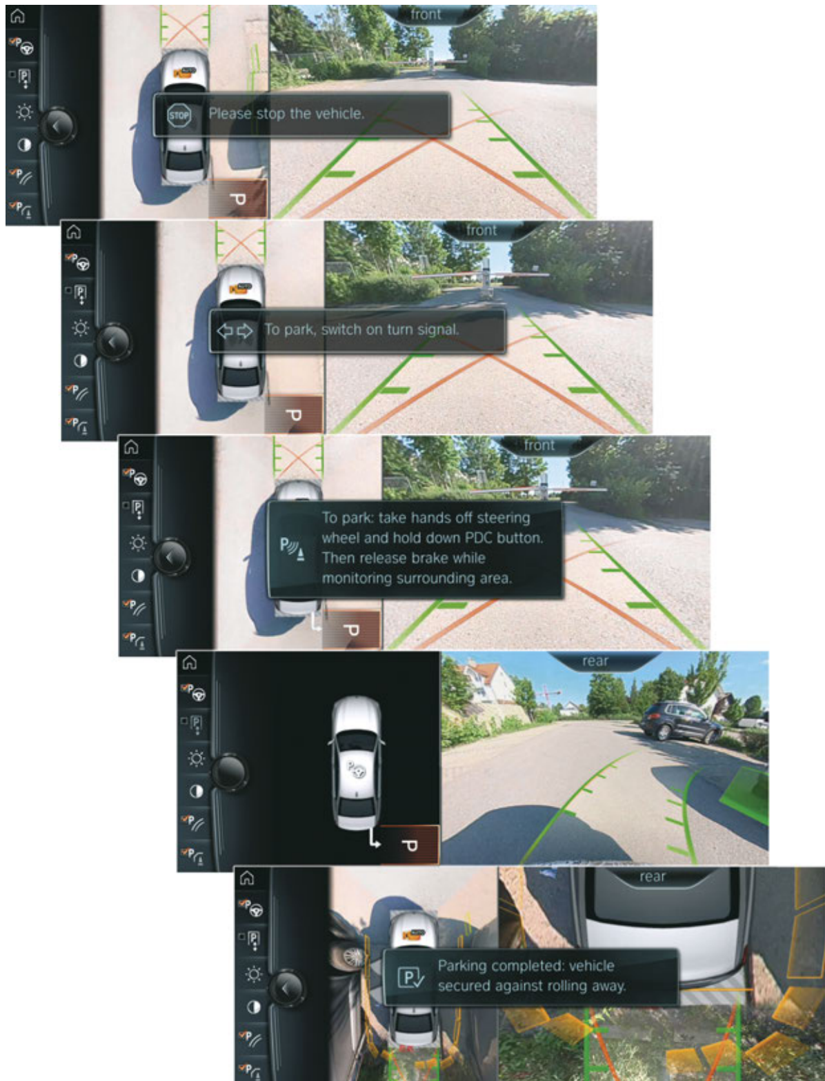
G12 parking procedure using PMA (bay parking)
