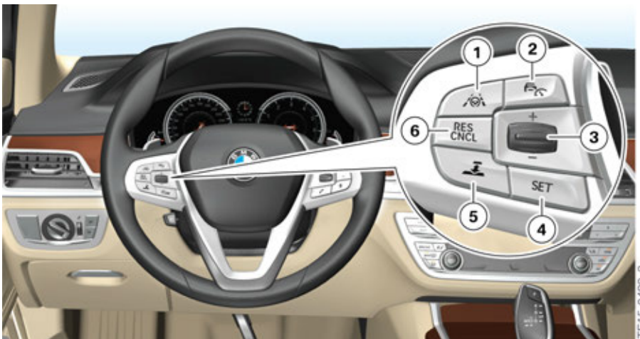
G12 buttons for ACC Stop&Go with Active Driving Assistant Plus II optional equipment (OE 5AT)
