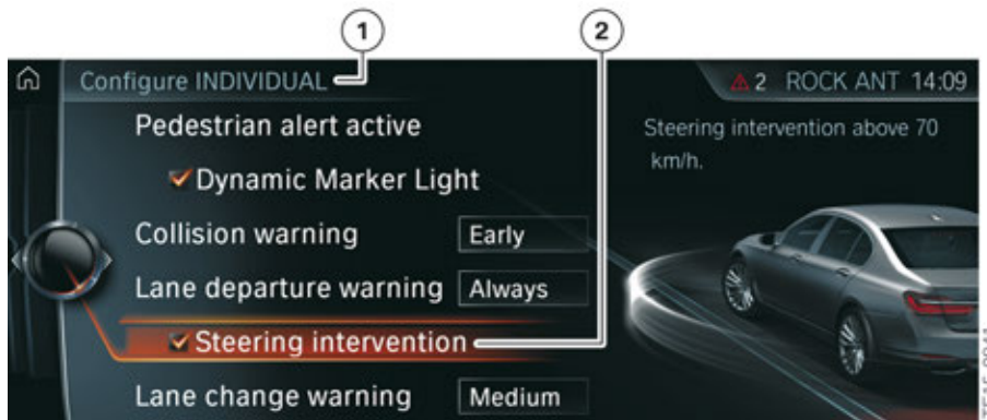
G12 Intelligent Safety view on the CID (lane departure warning with active steering intervention)
