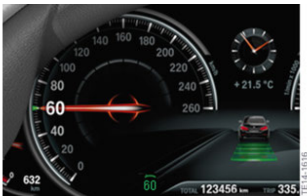
Displays in the instrument cluster when ACC Stop&Go is activated
