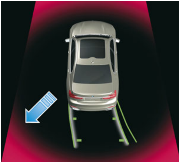
G12 cross-traffic warning in the PDC view
