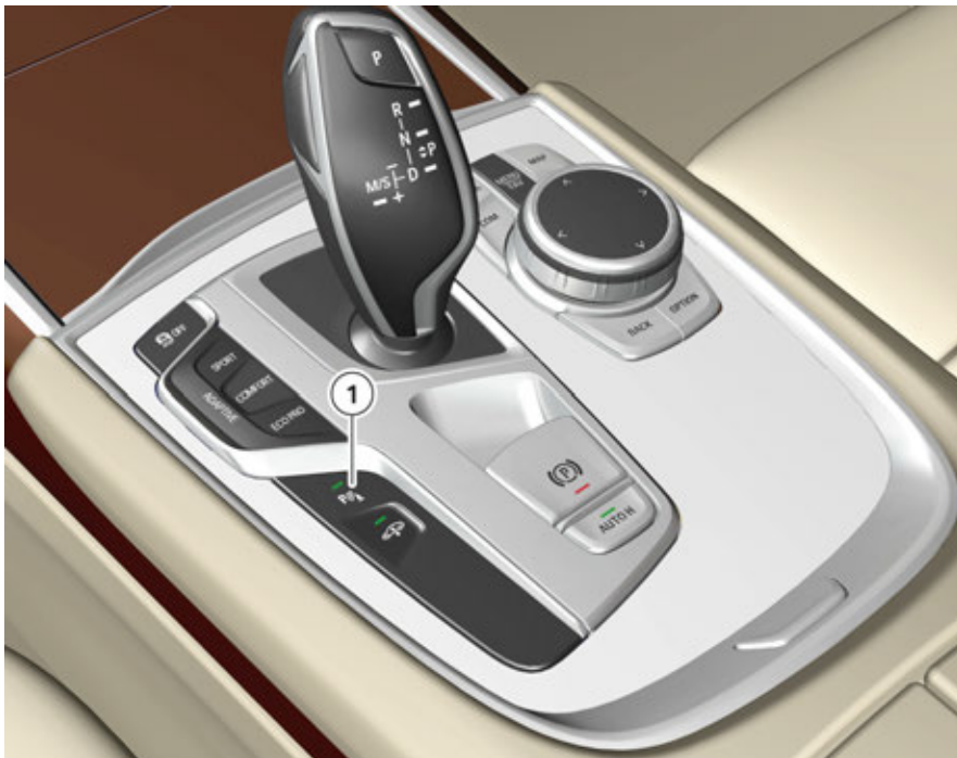
G12 switch block with parking assistance button
