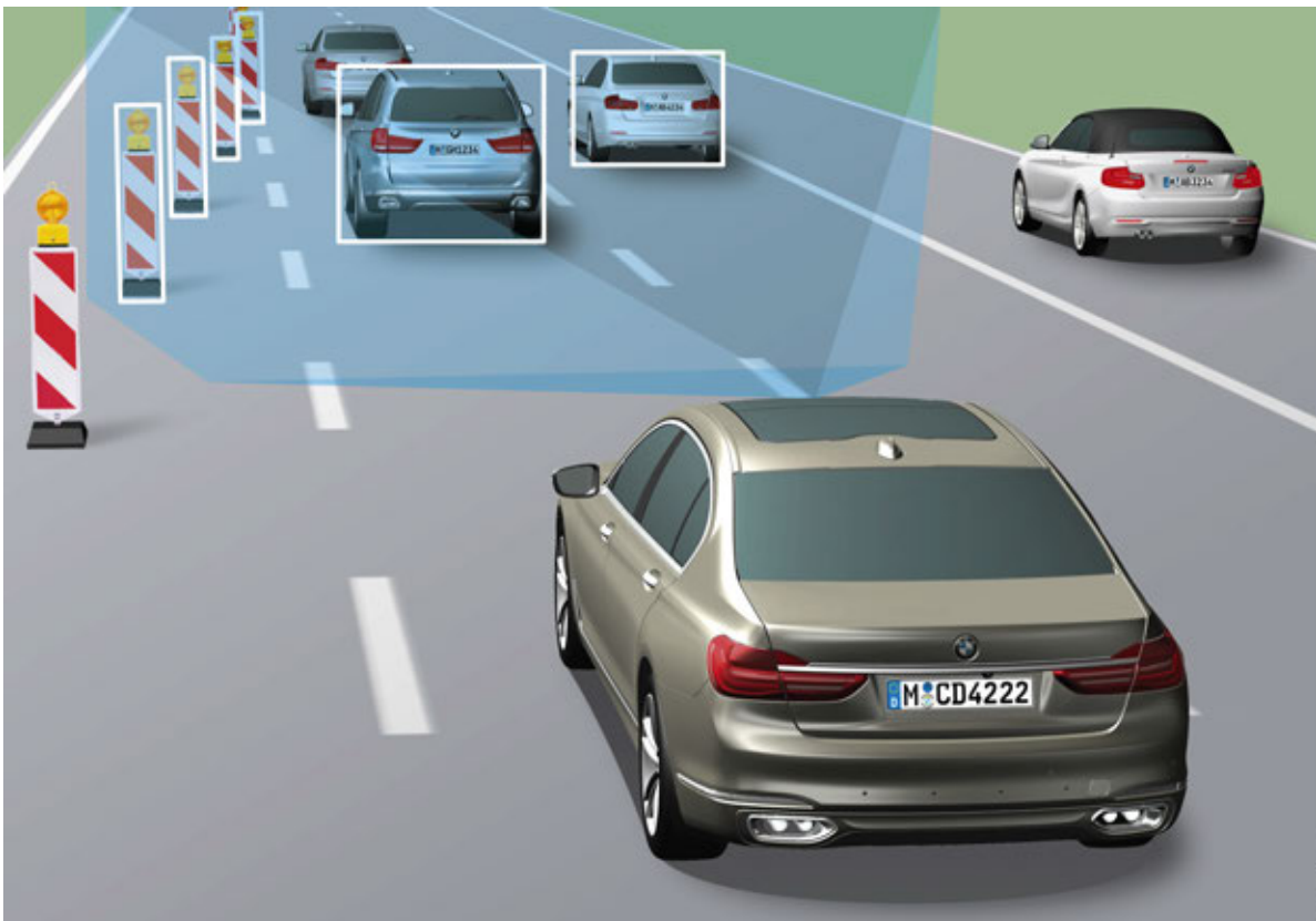
KAFAS stereo camera detection range
