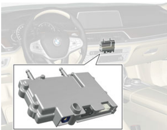
G12 Night Vision electronics (NVE) control unit
