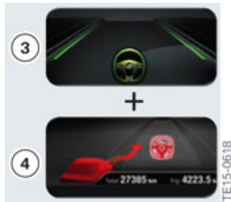
Overview of steering and lane control assistant including traffic jam assistant
