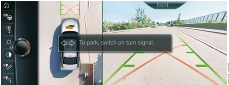
G12 parking procedure using PMA (parallel parking)
