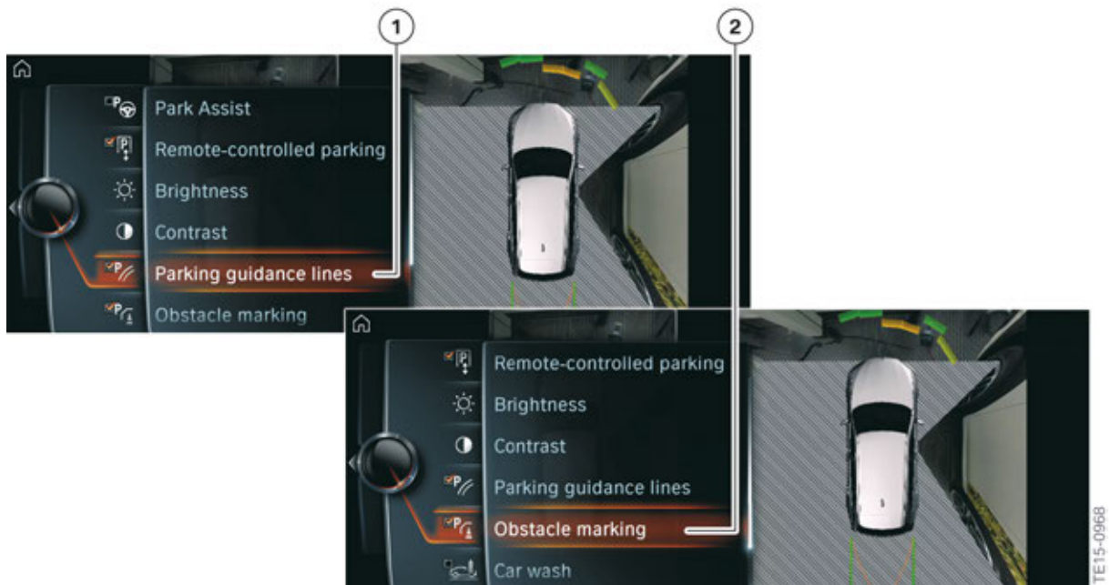
G12 configuration menu view for Obstacle marking and Parking assistance lines on the CID
