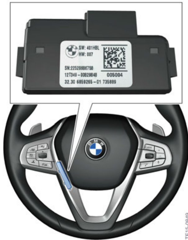
G12 steering wheel with touch detection control unit
