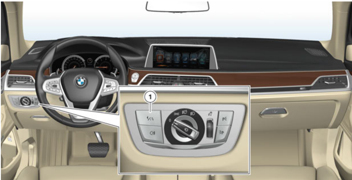
G12 button for thermal imaging camera/Night Vision
