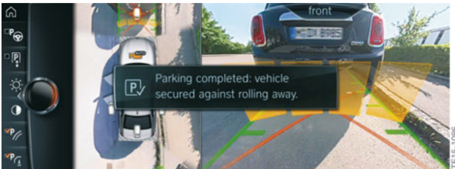
G12 parking procedure using PMA (parallel parking)
