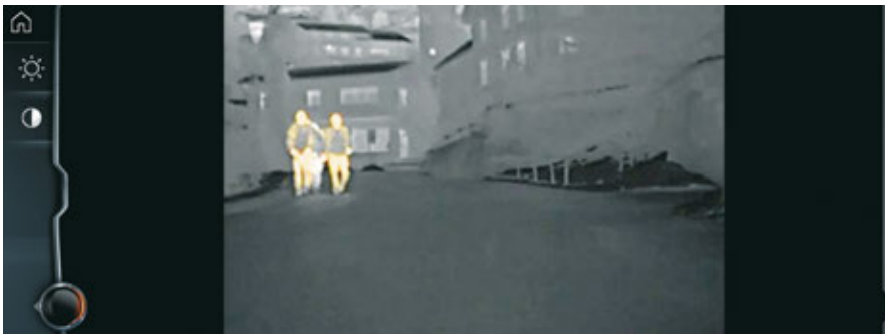
Night Vision camera image on the central information display showing detected people
