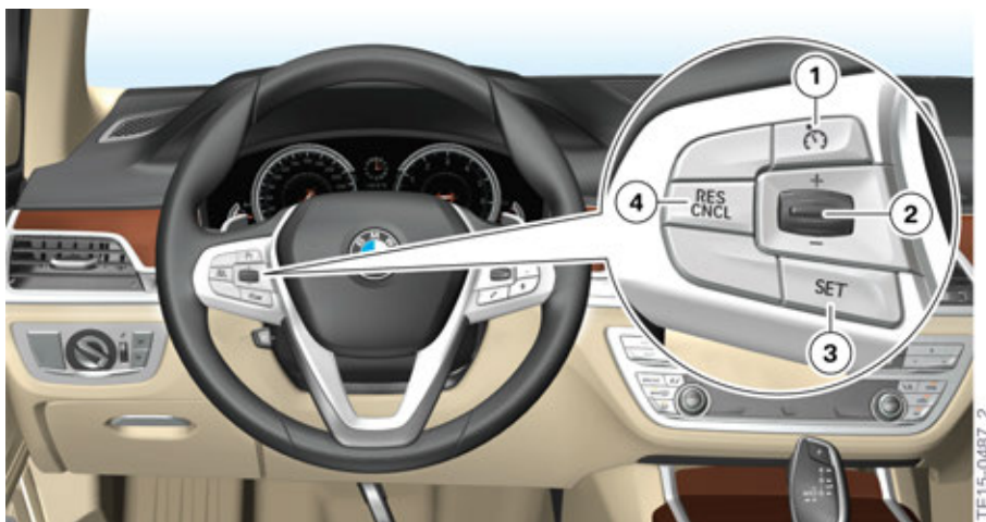
G12 Dynamic Cruise Control (DCC) buttons
