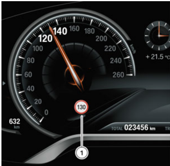
Top speed limitation symbol shown in the instrument cluster
