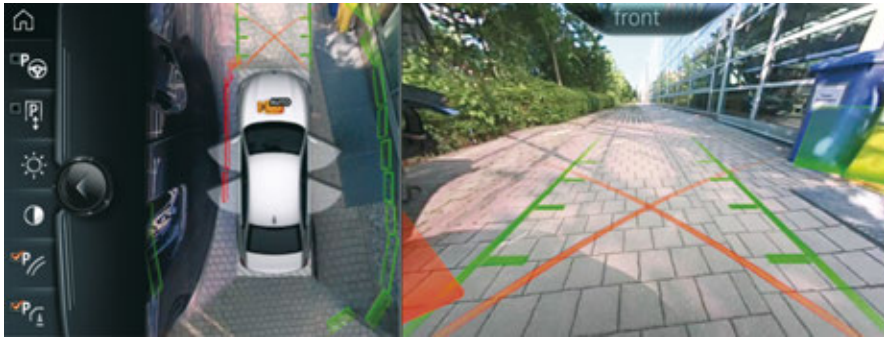
G12 door opening angle view on the CID
