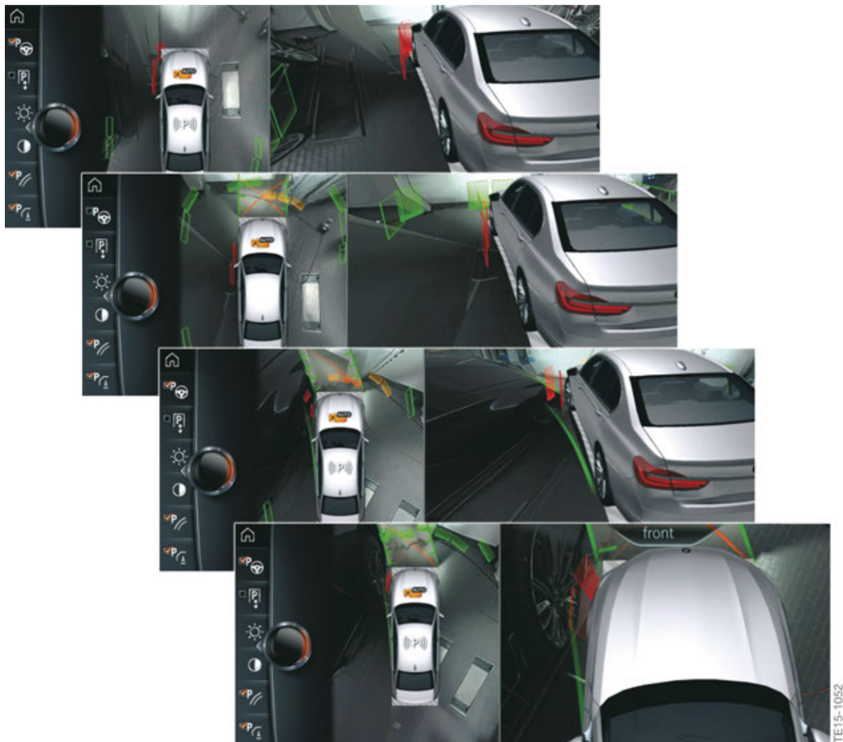
G12 side protection view (additional obstacle markings)
