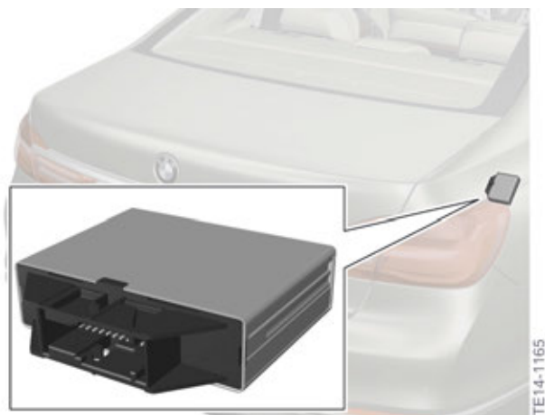
G12 control unit for Parking Maneuver Assistant (PMA)
