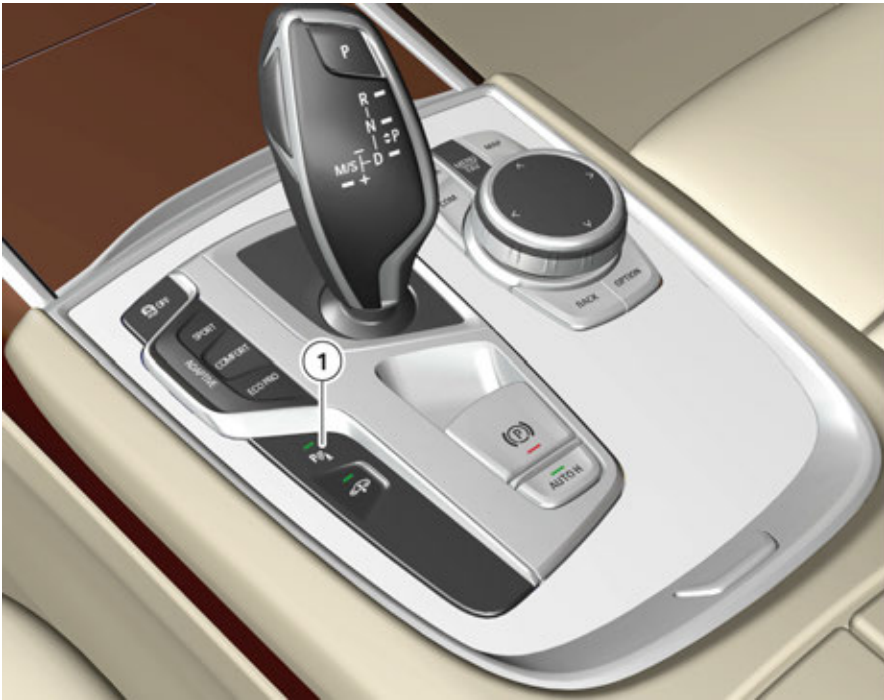
G12 switch block with parking assistance button
