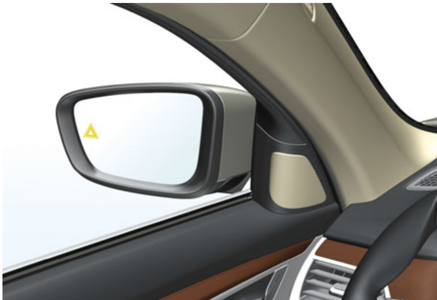
G12 signal unit (LED) in mirror glass
