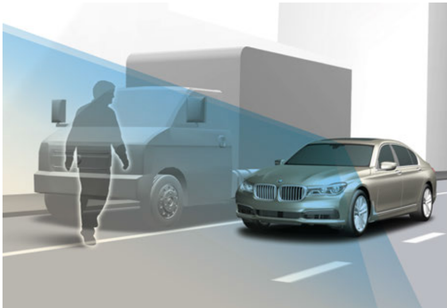
Example of pedestrian recognition by the KAFAS stereo camera: pedestrian approaching from the side steps into the road and is partially hidden
