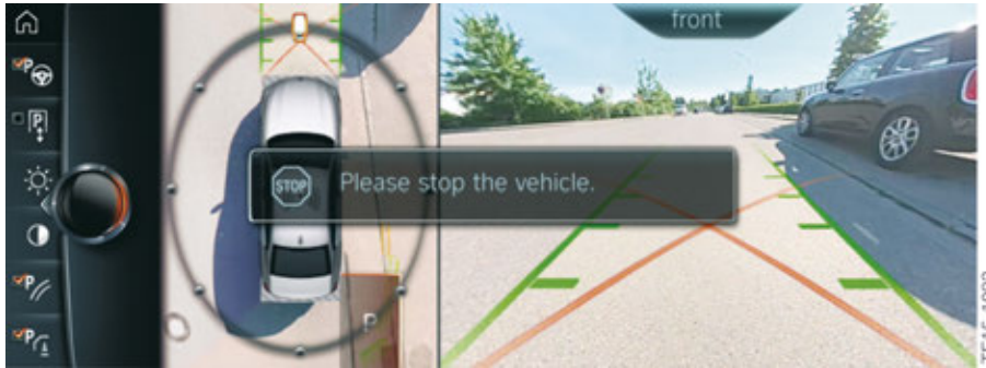
G12 parking procedure using PMA (parallel parking)
