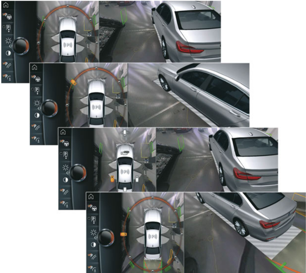
G12 exterior camera view (moving camera angle) on the CID
