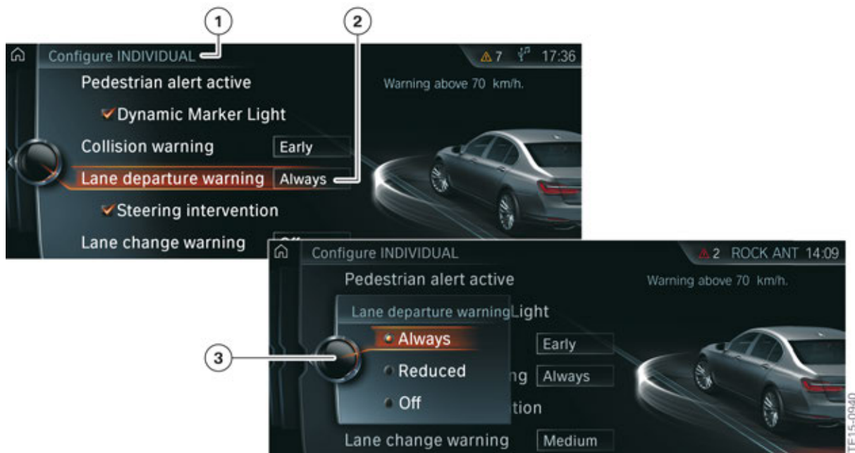
G12 Intelligent Safety view on the CID (lane departure warning)
