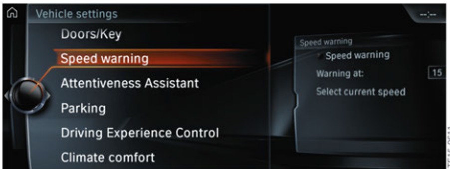
Speed limit warning display on the CID
