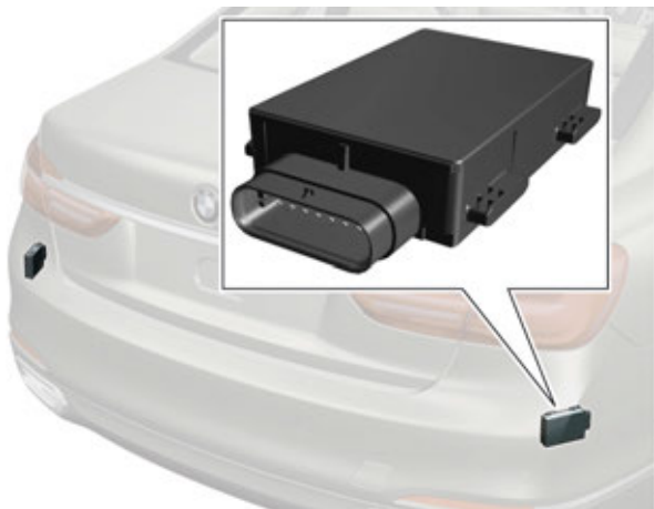
G12 Blind spot detection (SWW) (radar sensors)
