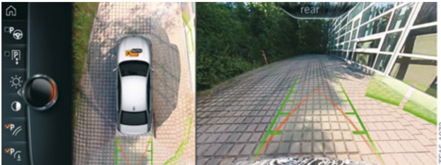
G12 rear view camera, view on the CID
