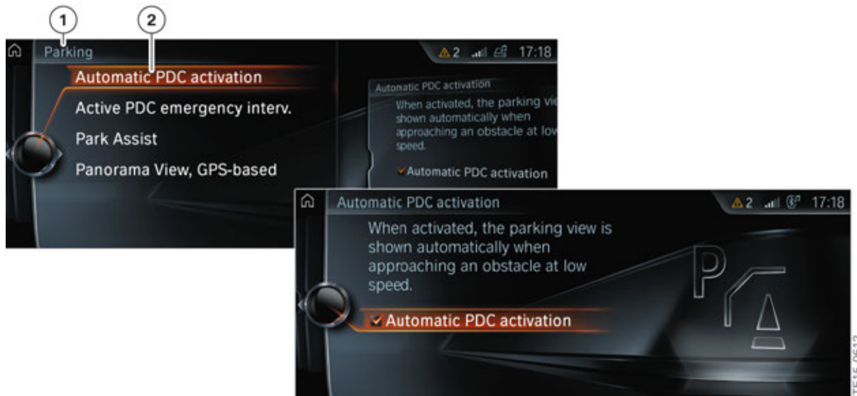
Automatic Park Distance Control on the CID
