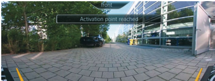
G12 automatic switch on at a set activation point
