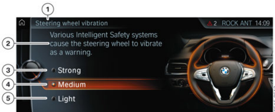
G12 steering wheel vibration settings menu on CID
