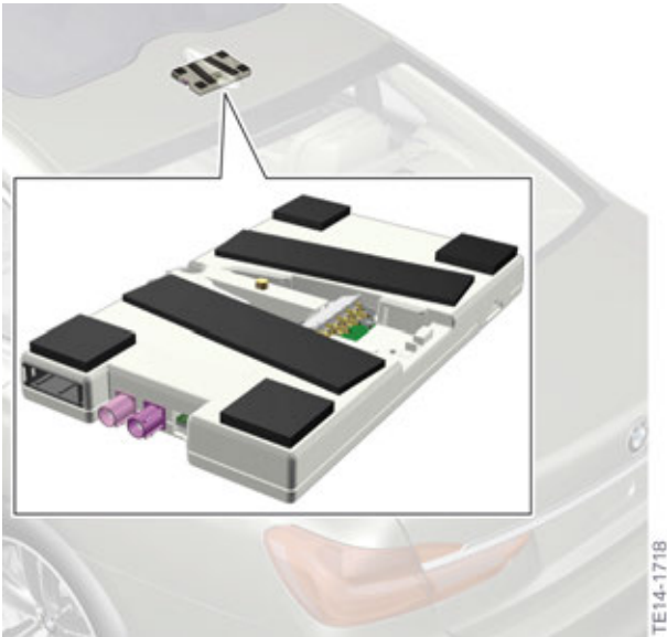
TCB2 installation location including the roof fin in the G12
