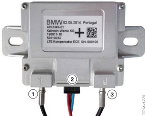
Line compensator in the G12
