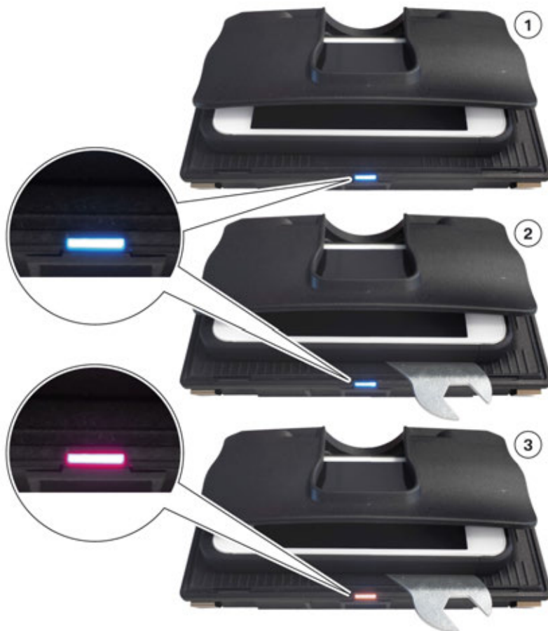
Charge status LED of the wireless charging tray
