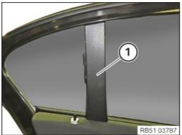
• Lever out trim (1) inwards with the special tool 0 496 569 (00 9 325) and remove it.
