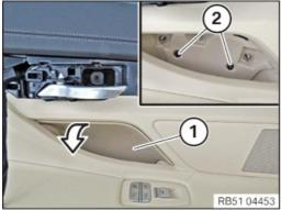
• In G12: Unclip the trim (1) in the direction of the arrow and feed it out of the door.
