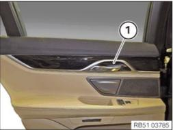
• Unclip the trim (1) with a suitable plastic wedge and remove.
