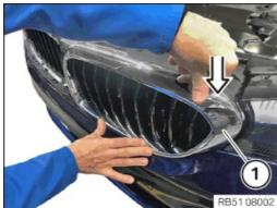
Press the front ornamental grille (1) in the area of the headlight in downward arrow direction, until lower latch mechanisms engage.
