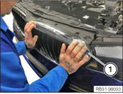
Press on all locking positions of the front ornamental grille (1) until all latch mechanisms are audibly engaged.
